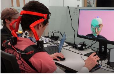
Fig. 6. (Top) Schematic of the experimental setup. (Bottom) The healthy subject performing a series of movements indicated by an avatar on the computer screen while wearing the Utah neck exoskeleton. Surface EMG was used to record the activity of the SCM and SC neck muscles.
